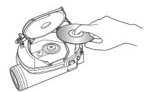
3 Push the section marked PUSH CLOSE on the cover of the disc compartment to close the cover.
