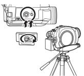
When the tripod is used, the card slot cover cannot be opened. Insert an SD card before attaching this unit to the tripod. (→ 35)
